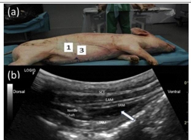
Figure 4: The meat phantom. It can be used for ultrasound guided TAP block needle guidance simulation.
